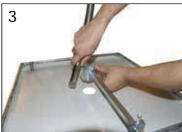
As seen in figure 3, the remaining 1/2" of the sprinkler line is fed to the middle clamp.
