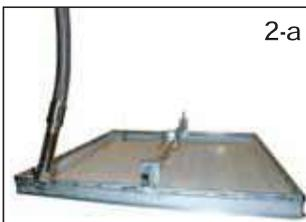
As shown in Figure 2-A, the box profile, right- and left-side supports and central clamp are joined. It must be noted that this measure is accurate only when there is no contact between the rotating and stationary components, i.e. in shaft-free conditions.
